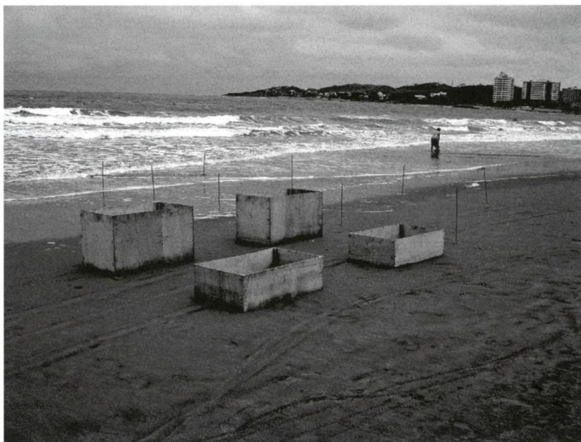
Picture 2.2.1 – Sampling protocol (beach of Playas). Wooden boxes are in place to hold the upcoming swash. In total, 8 boxes were used (only 4 shown) so 2x4 levels could be secured at the start of a sampling run (see text).
