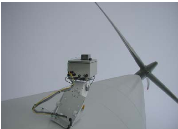
Figure 10. The TADS mounted on one of the turbines at the Nysted offshore wind farm. The pan and tilt head is set for vertical collision monitoring. Photo: Mark Desholm/NERI (adopted from Paper II).
