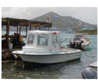
Figure 8.25. Bandit rigged boat - a type of commercial fishing vessel used to fish offshore for deepwater snapper and grouper in the U.S. Virgin Islands and capable of fishing to depths where deep water coral reside. Photo credit: Kojis 2005.
