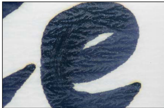
Figures 15 a and b. Permanent Marker OH. Close-up on writing on PE-bag after one year of exposure (left) and on reference sample (right)
