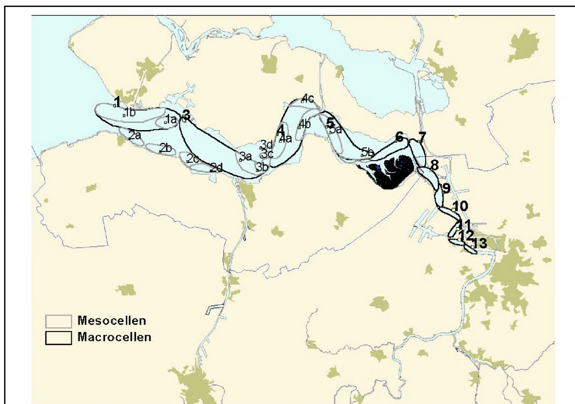
Figure. 3.12 Morfological schematisation of the Scheldt estuarium in morfometrical units.
