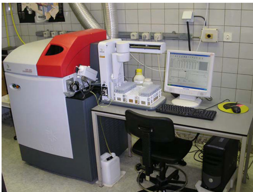
Figure 2.2. Varian Expert 700 quadrupole ICP-MS instrument.
