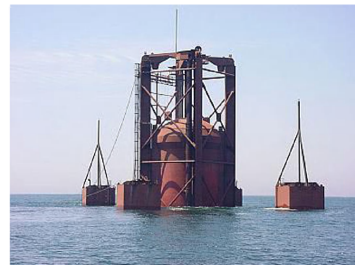
Figure 8 | The AWS device during the submergence process offshore Portugal (Teamwork Technology)
