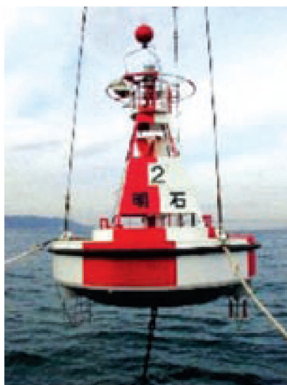
Navigation Buoy with Darrieus Turbine
