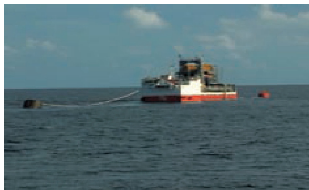
Floating Barge Mounted Plant and its mooring
