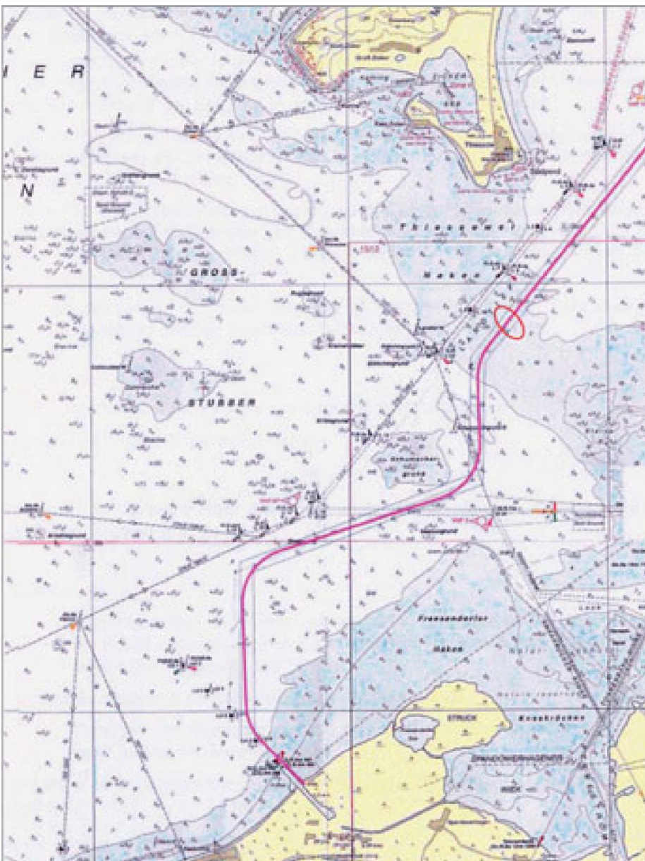
FIGURE 1: Map showing the planning of the pipeline and [the red dot] the ship that has to be removed. PICTURE: RGK
