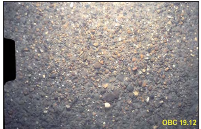
Photo 19.12: approx. 225 m from start of tow. Moderately sorted gravel on the surface with very little mud deposit.
