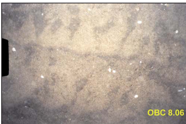
Photo 8.06: approx. 90 m from start of tow. A herring bone pattern in the small patches of settled floc. This implies that before slack water the near bed current was running along the line of the sand ridges rather than east-west across them.
