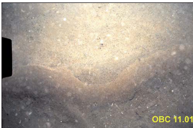
Photo 11.01: approx. at start of tow. Pronounced minor ripples in irregular and lingulate shapes, with some fine floc settled on the bed as well as suspended particles.
