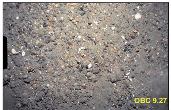
Photo 9.27: approx. 540 m from start of tow. A slightly higher proportion of sand on the heterogeneous gravel than most of the images from here.
