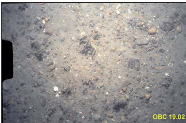
Photo 19.02: approx. 30 m from start of tow. Flat sea bed of embedded lag gravel with much mud that was easily disturbed. This photo was typical of much of the sea bed on this tow.
