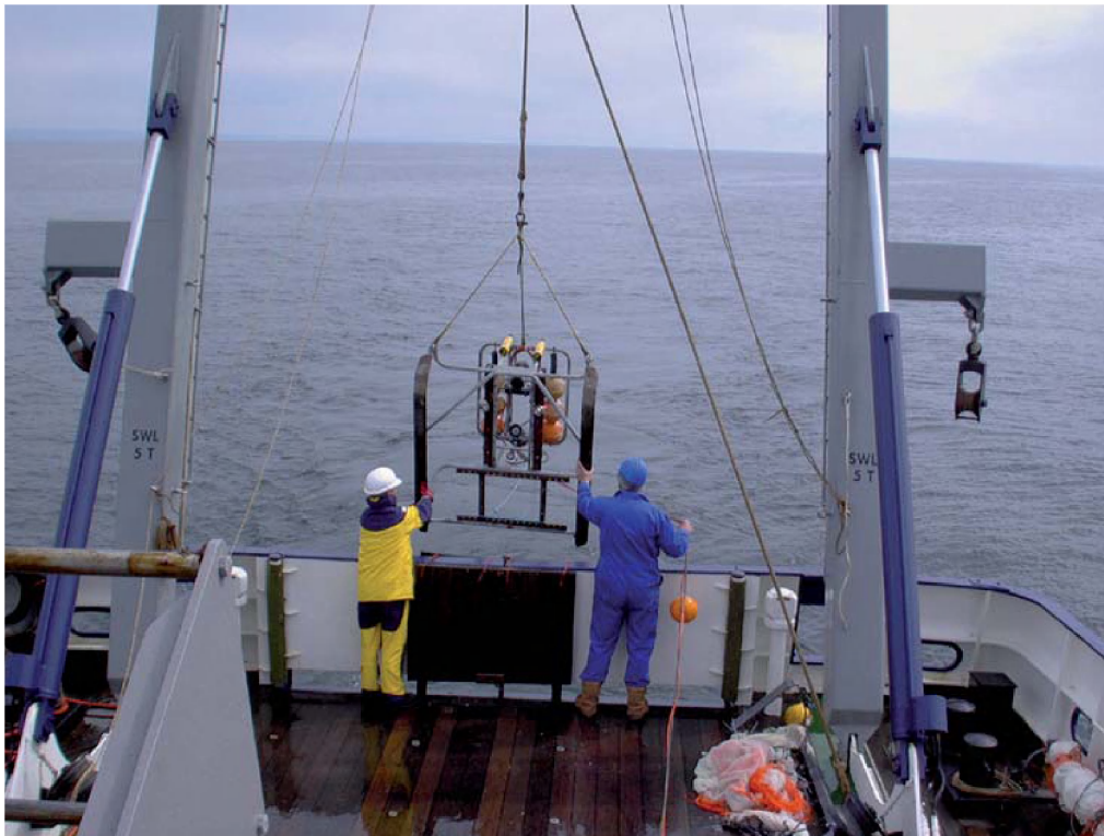
B. Deploying the camera sled. Note the yellow USBL range locating acoustic transducers attached to the sled on the May 2005 cruise.
