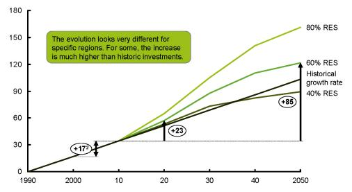
1 Development of grid is driven by the penetration of intermittent power sources (solar PV, wind onshore and wind offshore)
