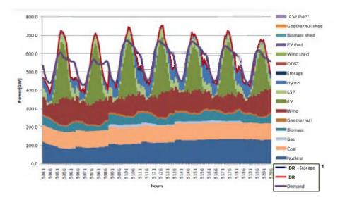
1 The graph shows how the original demand line (purple) is shifted to a higher level (red line) by DR to capture the higher PV production
