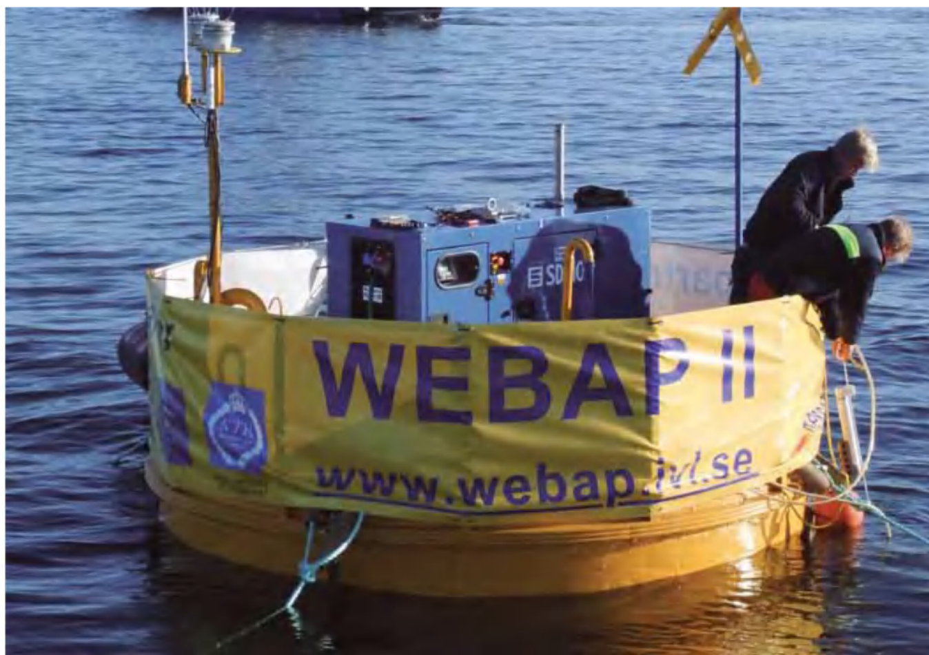
A wave-powered device - WEBAP - is being used for the aeration of coastal zones and open seas suffering oxygen depletion
