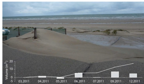
Figure 1 - Evolution of an experimental cross-shaped structure on the windward slope of the dike
