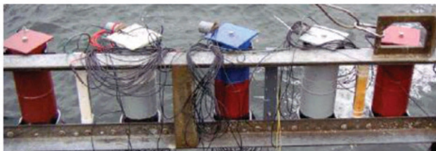
Fig. 8: Coated specimens for outdoor testing. Upper: Splash zone (SZ) specimens. Center: Intermediate zone (IZ) (originally without scribe, no effect after 13 months; scribe added after 13 months to produce mechanical damage to the systems.) Bottom: Underwater (UZ) specimens Courtesy of the authors
