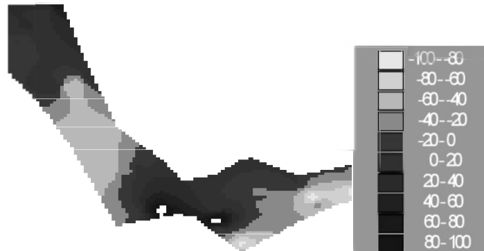
Figure 4 – Difference in percentage of electrical resistivity distribution between 2003 and 1967 investigation campaigns with Schlumberger array AB = 60 m
