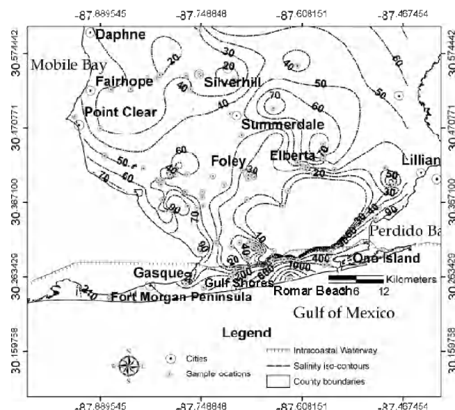
Figure 1. Aquifer zone A2- salinity concentration map. Concentrations are in mg/L; contour lines are labeled correspondingly.
