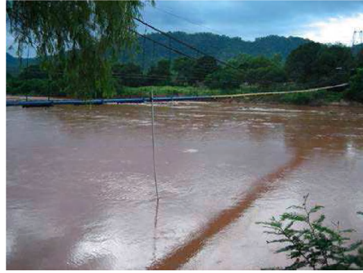
Figure : Installation of the limnimeter in the Rio Parapeti. The pressure probe is inserted into the pole.
