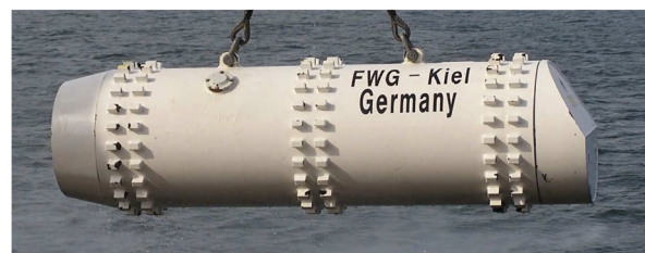
Figure 2. BRM, length: 1.70m, diameter: 47cm, weight: 5.0 kg. Bow ring at the right side (Wever et al. 2004).
