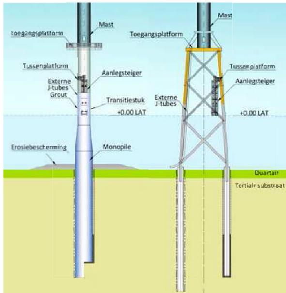
Figure 2: Monopile (left) and jacket foundation (right) (source: Technum-IMDC)
