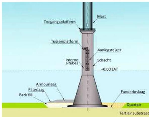
Figure 3: Gravity Based Foundation (GBF) (source: Technum-IMDC)
