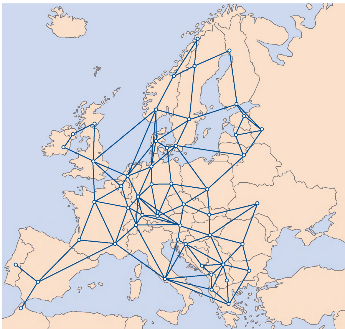
FIGURE 12.3: OFFSHOREGRID ZONES IN THE EUROPEAN GRID MODEL FOR THE HUB BASE CASE 2030
