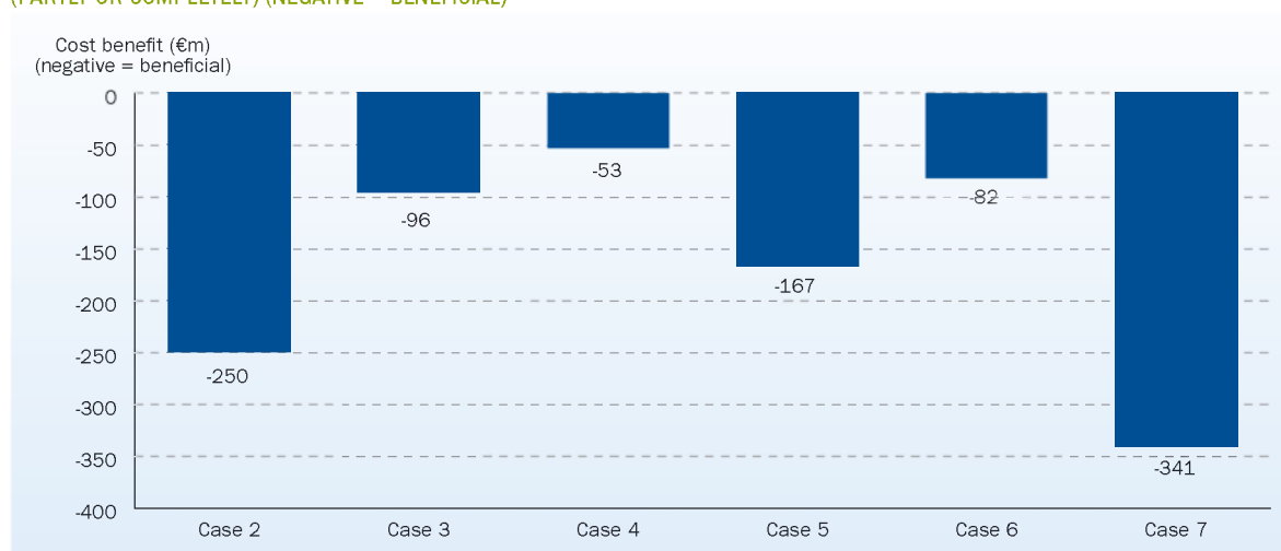
FIGURE 4.20: COMPARISON COST-BENEFIT OBTAINED BY INTERCONNECTING A GERMAN WIND FARM INTO THE COBRA CABLE (PARTLY OR COMPLETELY) (NEGATIVE = BENEFICIAL)
