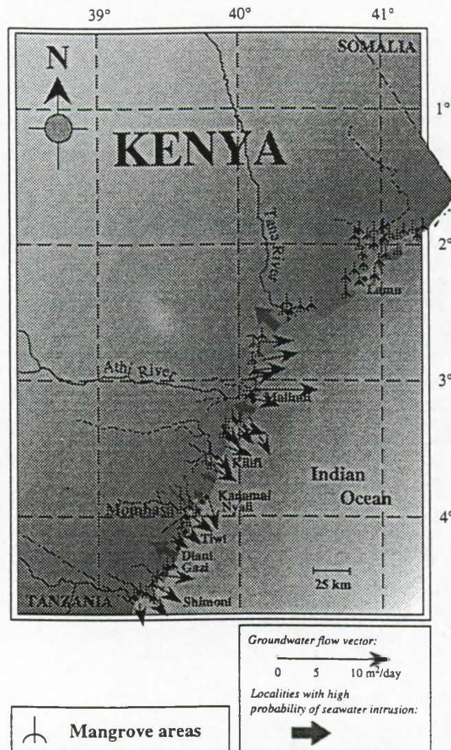
Figure 8. Groundwater flow: graphical output (vectorial) of the modelled situation along the Kenyan coast between the Tanzanian border and Tana River when 350.000 m 3 /day is pumped at Mzima springs. Only those areas with groundwater flow higher than 1 m 2 /day and regions with a high probability of seawater intrusion are indicated.
