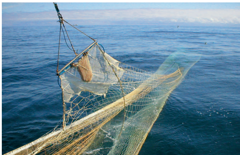
Pelagic mid-water trawl, typically used in herring and mackerel fisheries
