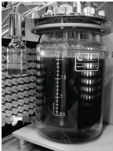
Figure 5 - Lab-scale CSTR photobioreactor used in the experiments.
