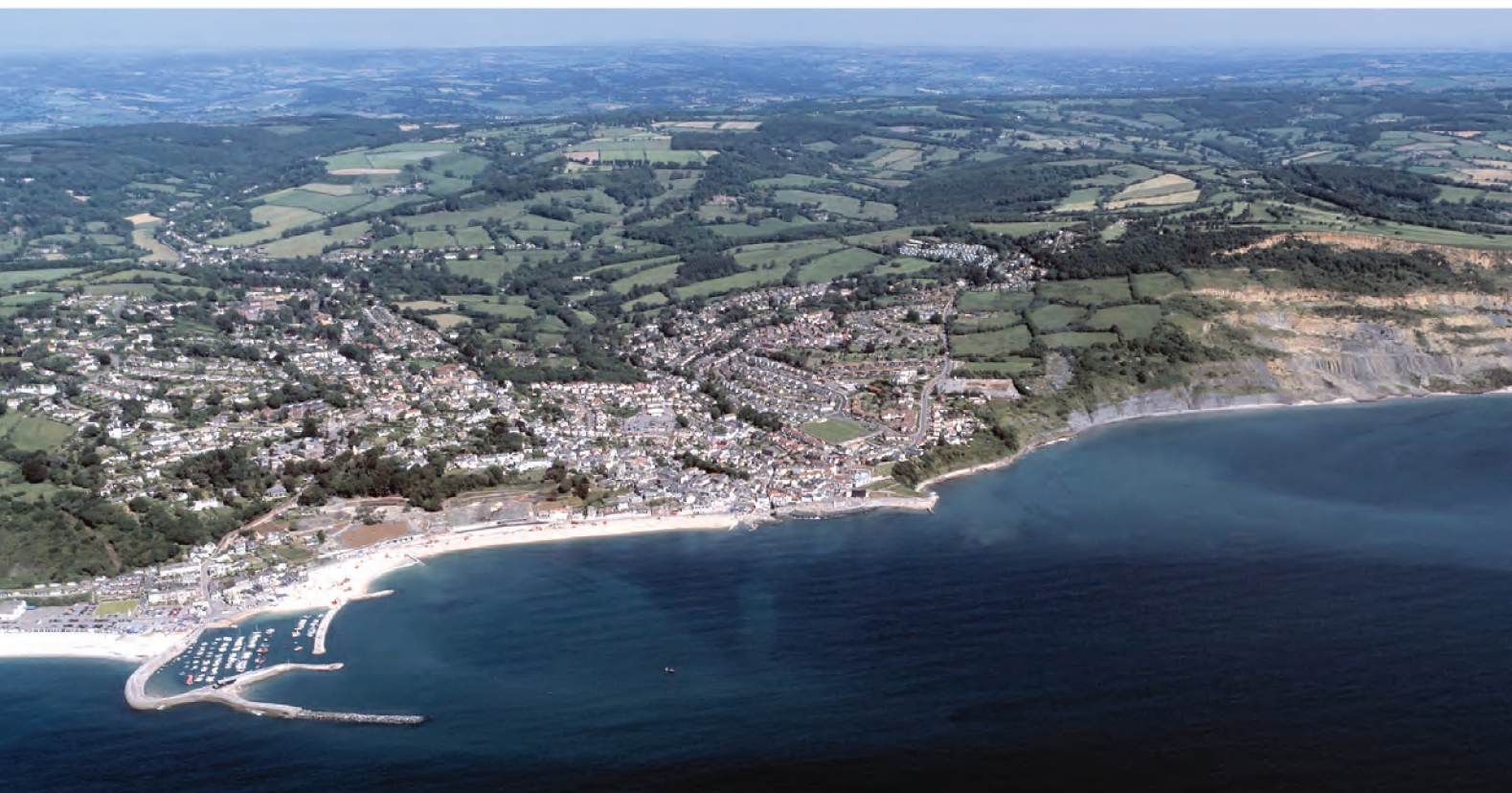
Plate 3.1: The historic coastal town of Lyme Regis in Dorset, UK was developed on a landslide complex. Following detailed studies and ground investigations a major programme of coast protection works and slope drainage has been implemented to reduce erosion and landslide risk. Further works are under consideration for the frontage to the east.
