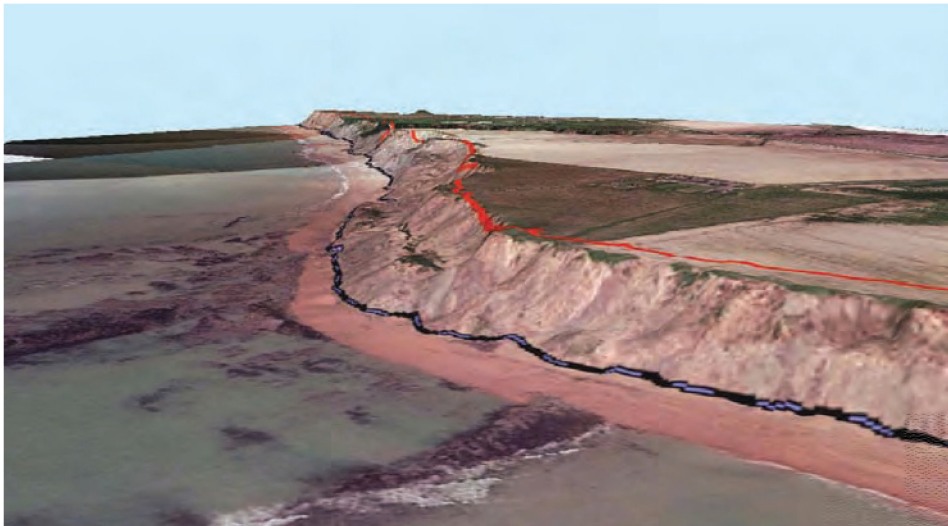
Figure 6.8: Simulation of cliff base recession of a fifty year timescale for part of the south-west coast of the Isle of Wight, UK.
