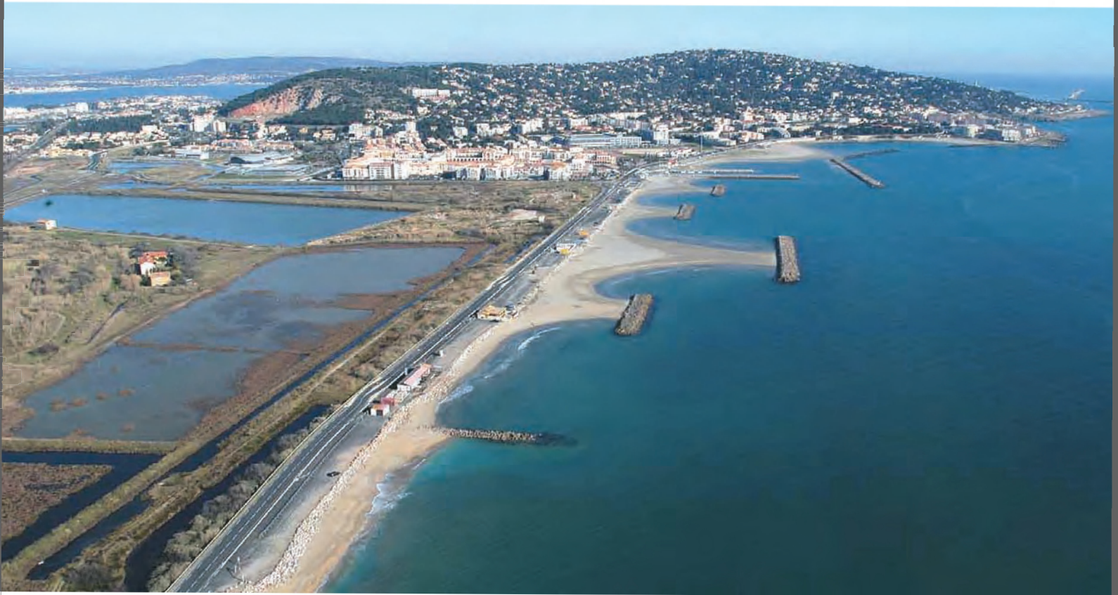
Plate 2.6: Part of the low-lying coastal zone near the town of Sete within the Languedoc-Roussillon Region of France. The barrier beach (lido system) protects assets, and lagoons of environmental importance from coastal erosion. Coastal protection works also reduce risks to the highway from marine erosion.
