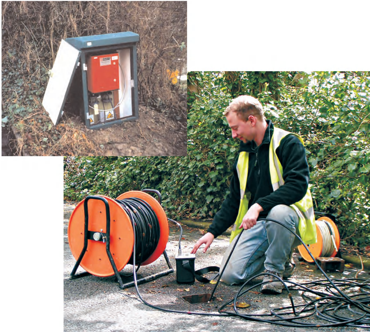
Plate 4.2: Taking inclinometer readings in the Ventnor Undercliff, Isle of Wight; a datalogger (inset) gathers ground movement data which can be downloaded to assist landslide risk management.
