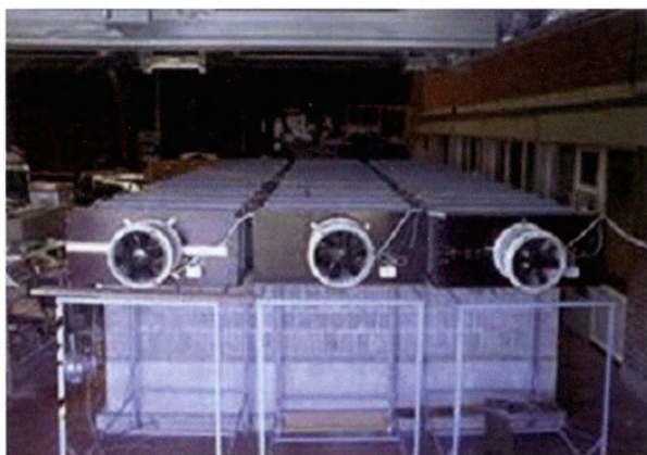
Figure 4. Test installation for ammonia emission measurements
