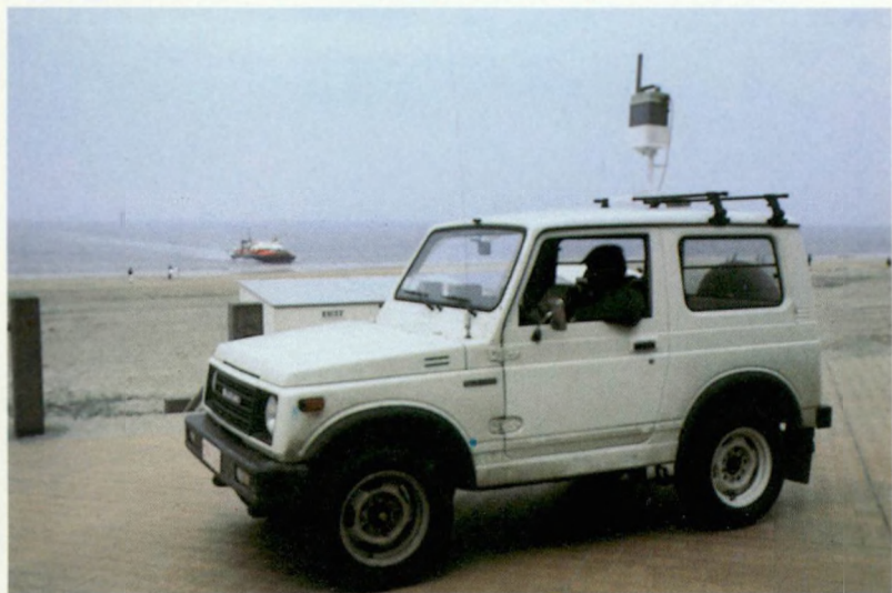
fig. 14 : removable Trisponder beacon mounted on a jeep
