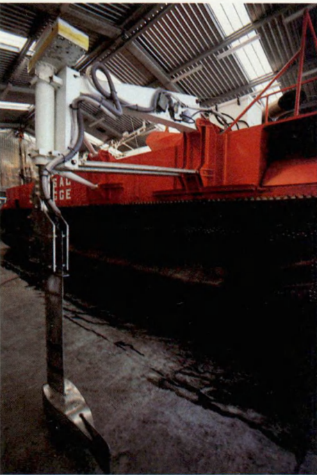
fig. 7 : hydraulic retractable arms with sword and fish.
