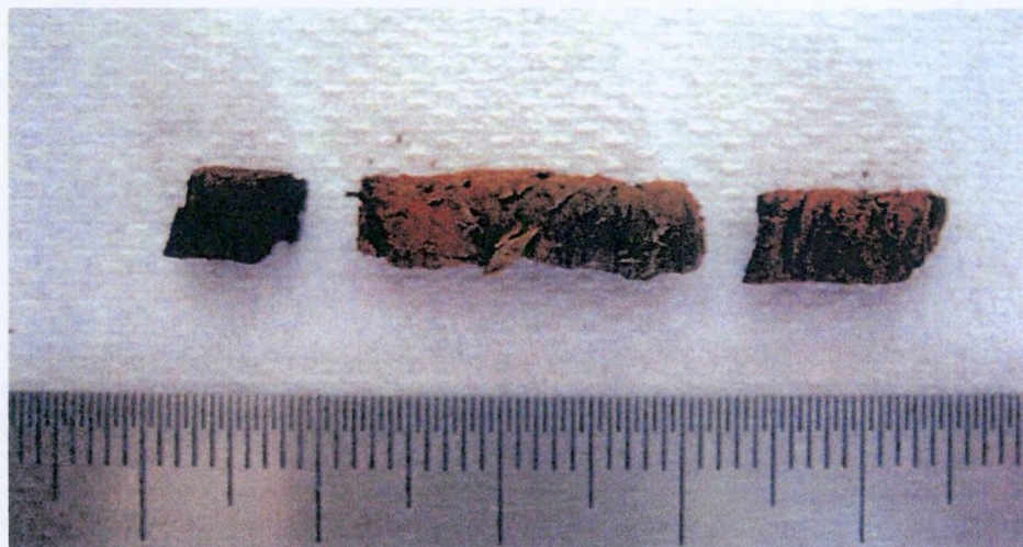
Figure 4: Section of wood core after determination of density. The outer surface of the wood (i.e. exposed to seawater) is to the left of the picture.
