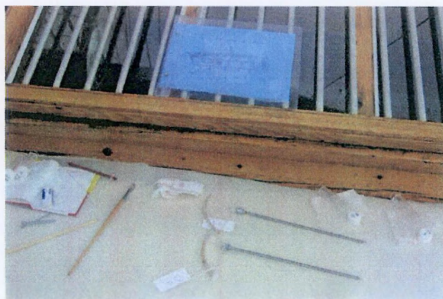
Figure 16. The field laboratory at "Anna Rogde". Needles have been prepared for the next core sampling, the labels indicating that the next samples are to be collected from spot 3B and 3C. The plastic vials are prepared to hold core samples from the spots 4B and 3A.
