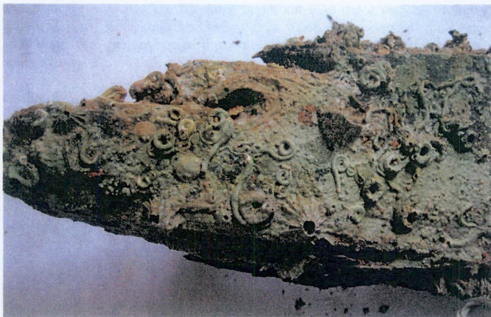
Figure 6: Biofouling organisms on the surface including calcareous tubeworms and barnacles.
