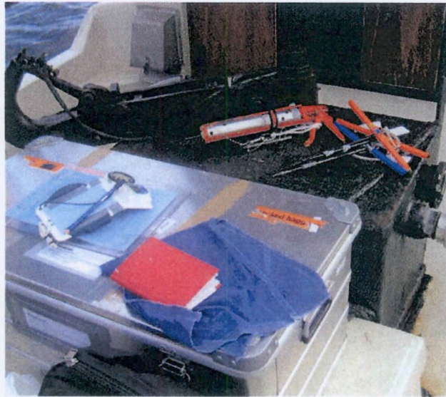
Figure 15. The field laboratory at "Astrid". On the black table are the Pilodyn (to the left) and the three corers. The aluminium suitcase holds the rest of the laboratory.
