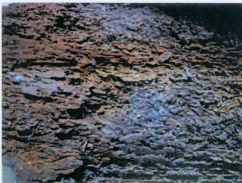
Figure 7: Surface of wood sample extensively degraded by wood boring crustacea.
