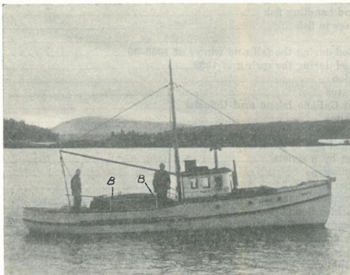
Fig. 1. Boat fitted with bait-tank as used in tagging herring. (B) Bait-tank.
