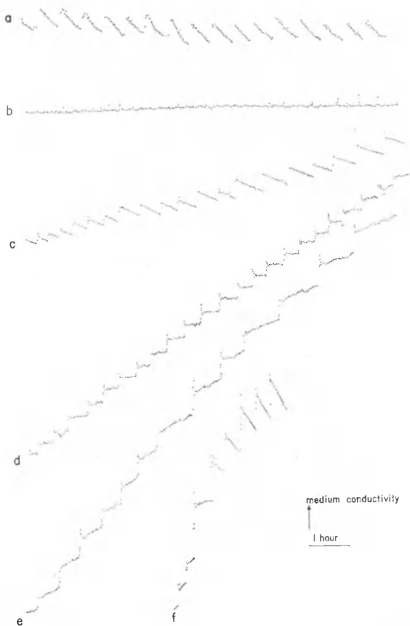
Fig.6. Examples of conductivity changes registered for C. crangon (on a different scale for the individual registrations); a, conductivity changes in a hypo-osmotic medium, salinity of medium ( S_m ) the same as to which the animal had been adapted ( S_m = S_a = 7\text{‰} S); b, conductivity in a hyperosmotic medium ( S_m = S_a = 36.3\text{‰} ); c, conductivity changes after transfer to lower salinity in a hypo-osmotic medium ( S_a = 12.1\text{‰} , S_m = 7.3\text{‰} ); d, as c ( S_a = 20.7\text{‰} , S_m = 11.1\text{‰} ); e, as c ( S_a = 20.7\text{‰} , S_m = 11.1\text{‰} ); f, as c ( S_a = 12.1\text{‰} , S_m = 7.3\text{‰} ). Temperature 21^\circ\text{C} .
