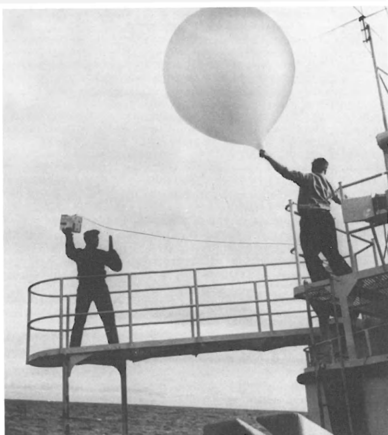
Figure 6 Release of radiosonde balloon from an oceanic weather station
