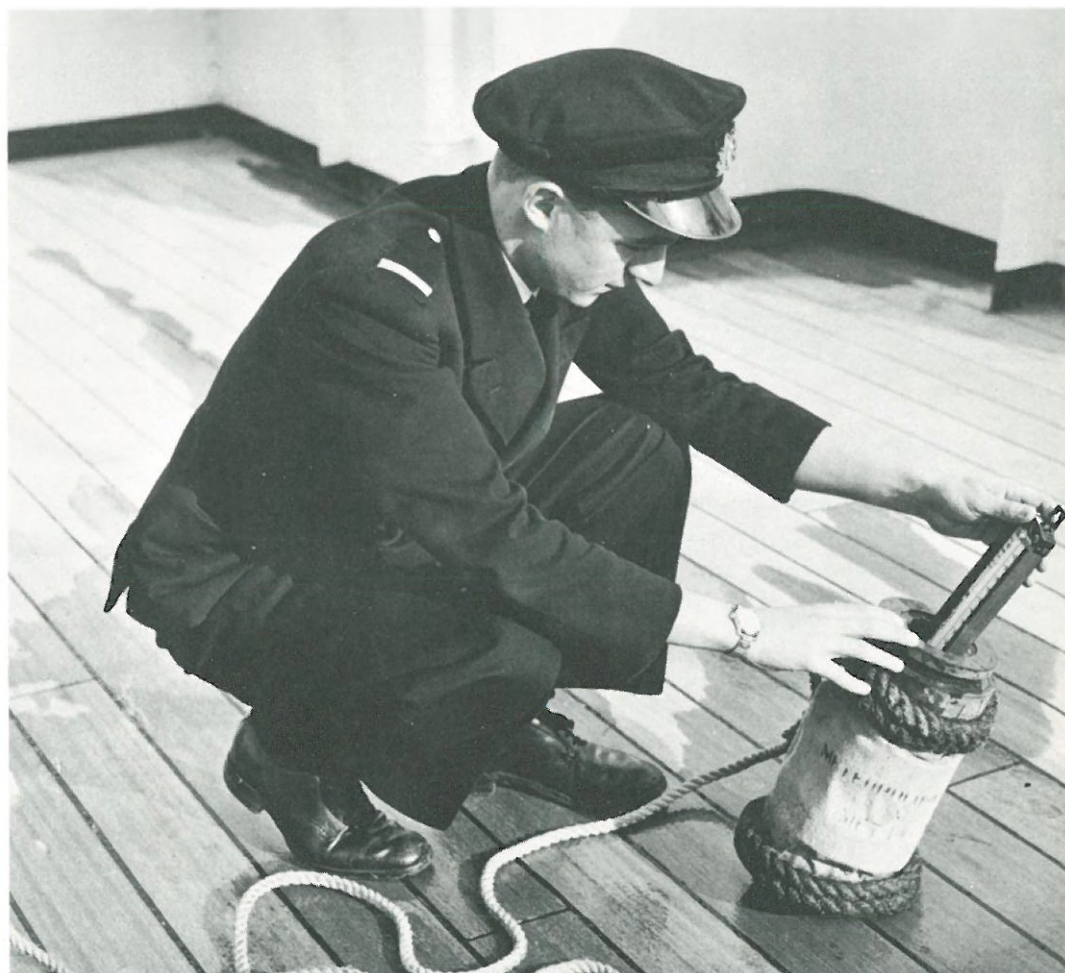
Figure 9 Measurement of sea surface temperature by bucket method
