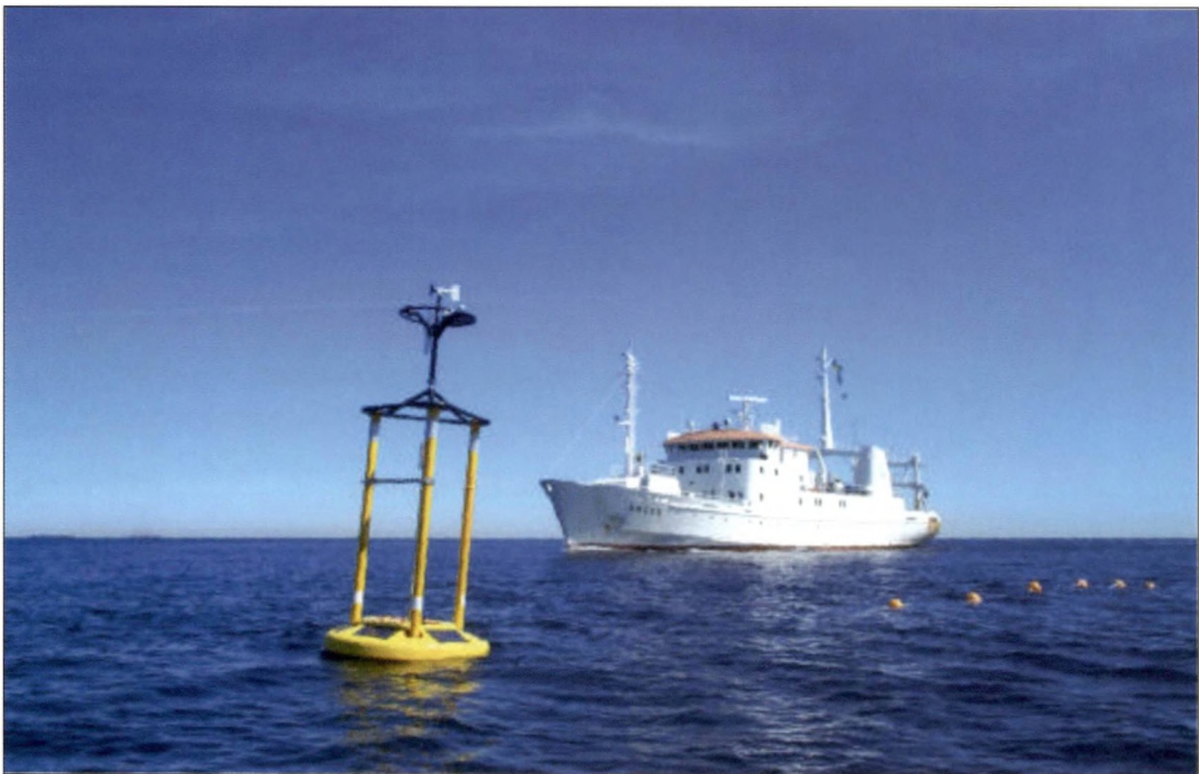
Figure 2.2 To support operational modelling, the exchange of water and substances between the Baltic and the North Sea is monitored continuously by a network of oceanographic buoys and by frequent (> 25/year) monitoring cruises in the transition area. (The exchange monitoring is a Danish-Swedish contribution to the HELCOM environmental monitoring programme, COMBINE)
