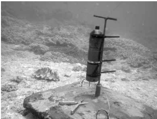
Plate 1. VR2(W) acoustic receiver in position at an aggregation site.
