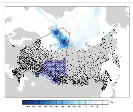
Figure 1. Map showing the positions of the 820 snow cover stations (black dots), with the Barents/Kara Sea (BKS) and the 'southwestern Siberia' regions highlighted (red frame and blue crossing, respectively). Blue shading shows the composite of HadISST October and November sea-ice concentration anomalies of low minus high sea-ice years.
