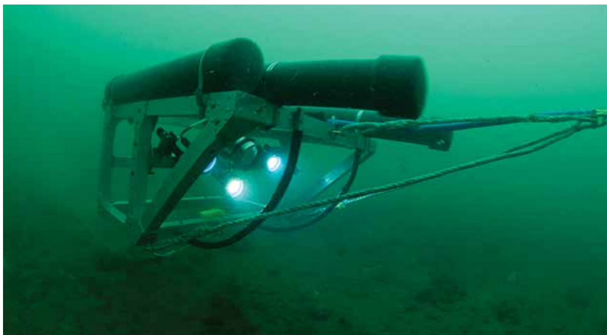
Fig 2.5 Underwater image of a new 'flying array' towed camera system that minimises contact with the seabed. From Sheehan et al. (2010). Courtesy of Prof Martin Attrill.
