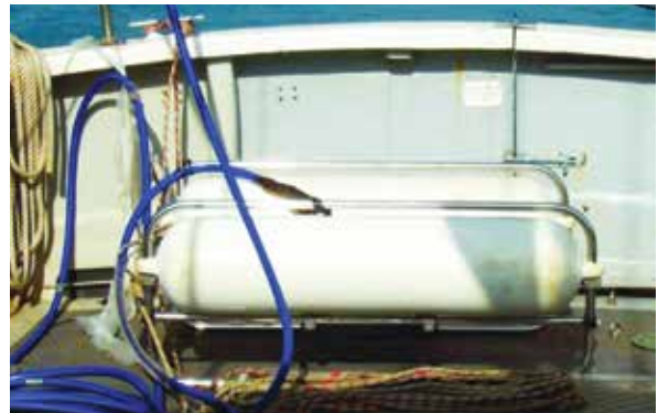
Fig 5.5 Boomer sub-bottom profiling equipment. Courtesy of Wessex Archaeology.
