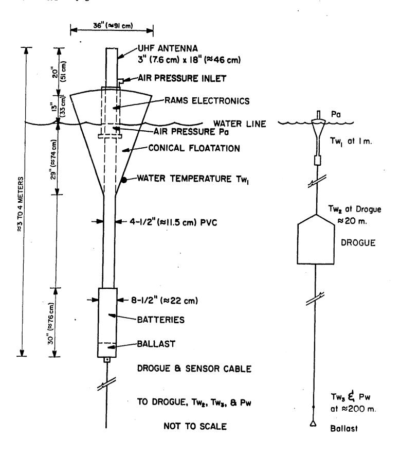
FIGURE DRIFTING BUOY UNDER DEVELOPMENT AND TEST
