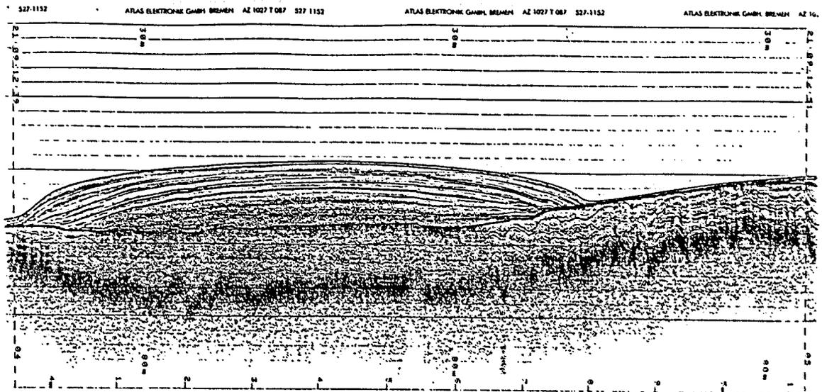
Figure 3. Vertical section through western margin of basin F41 in S - N (left to right) direction, 1 NM. Till at the bottom of section (thick black zone) is overlain by younger and recent fine sediments. Compare with figure 2a.
