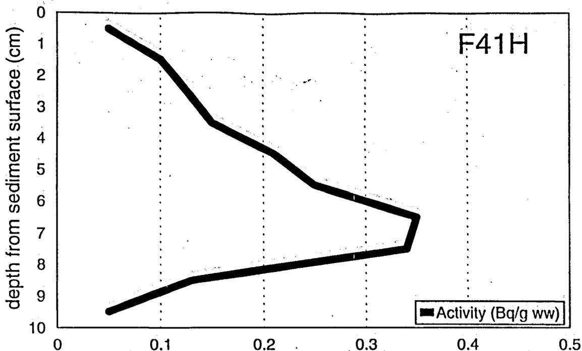
Figure 4.  $^{137}\text{Cs}$ -activity profile from sediment core at site F41H.
