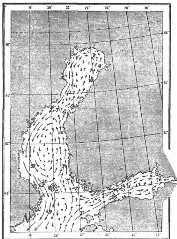
Fig. 2 Chart of the average horizontal surface currents in the northern Baltic area. 1 mm vector length corresponds to a current velocity of 0.5 cm/sec. The stability of the currents is indicated by the numbers 0—100. 100 stands for current with unchanging direction of flow, 0 for current returning the water particle to its original point of departure. (Palmén 1930.)
