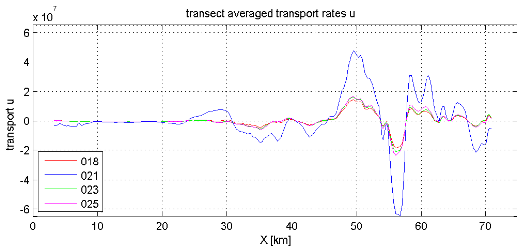
Figure 3.17 Computed longitudinal transport from the various runs (in \text{m}^3/\text{s} per transect cross-section width)
