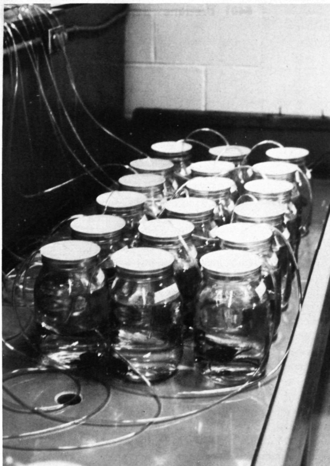
Figure 1.—Exposure system for short-term static tests.
