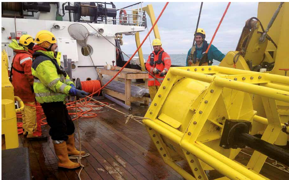
VLIZ HAS A VIBROCORER which can collect cores of up to 3 m long. The instrument is used aboard RV Simon Stevin.
