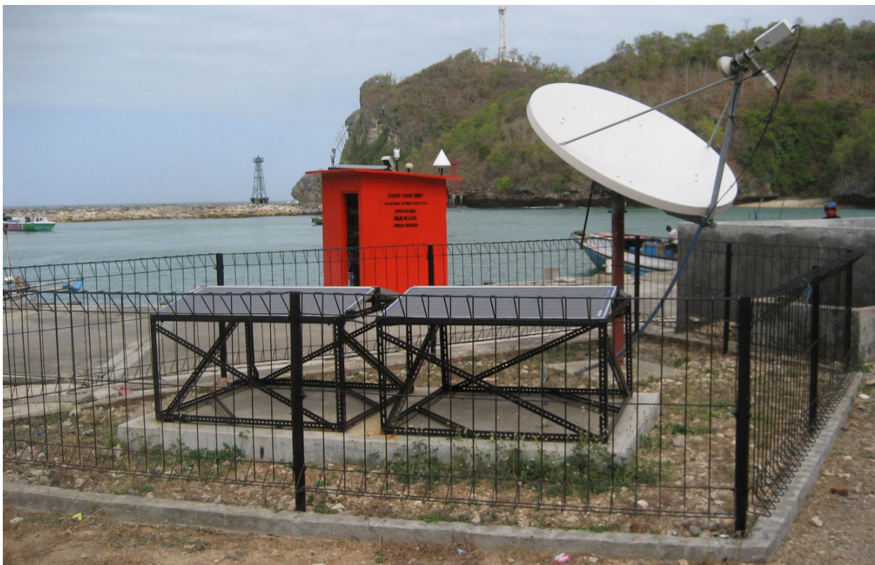
Figure 7.5 A VSAT dish alongside a tide gauge in Indonesia. This station is also equipped with an OTT Kalesto radar gauge and GPS receiver. (Photograph Tilo Schöne, GFZ).
