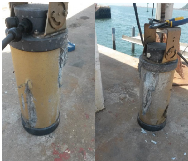
Figure 2. Durban's transducer showing corrosion damage.
