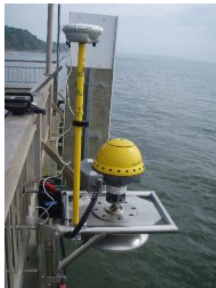
Figure 3. GPS survey of WaveRadar REX on Teignmouth Pier ©Teignbridge District Council.
