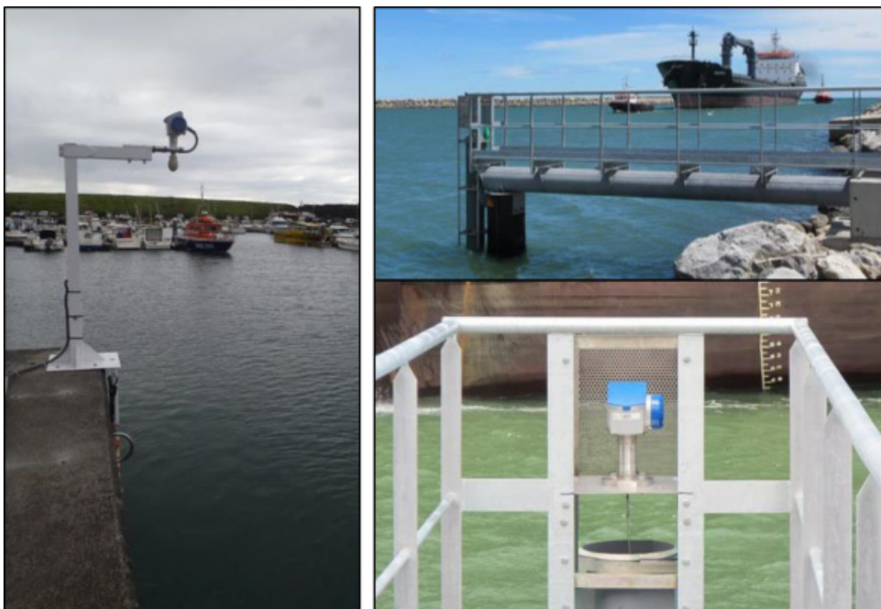
Figure 3. Examples of RONIM tide gauge installations : Optiwave mounted in open air at La Réunion (left) and Optiflex mounted in a PVC stilling well at Port-La-Nouvelle (right).
