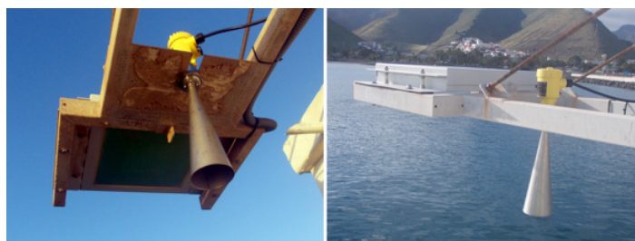
Figure 5. Installation of a VegaPuls62 radar beside the Miros permanent sensor for in-situ verification during routine annual maintenance visits.
