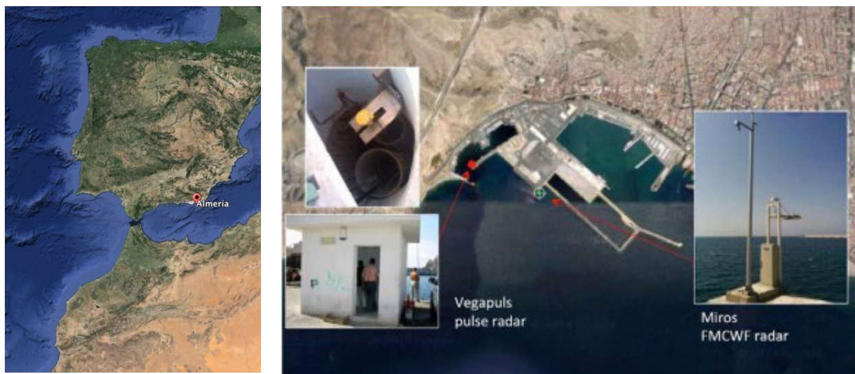
Figure 6. Position of the two radar sensors in Almería: VegaPuls (pulse radar) from IGN and Miros FMCW radar from PdE (REDMAR).
