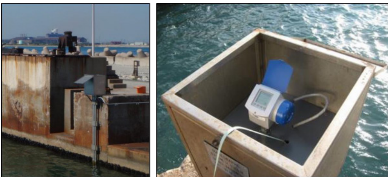
Figure 4. Example of RONIM tide gauge installation. Optiwave mounted in stainless steel stilling well at Fos-sur-Mer (right).
