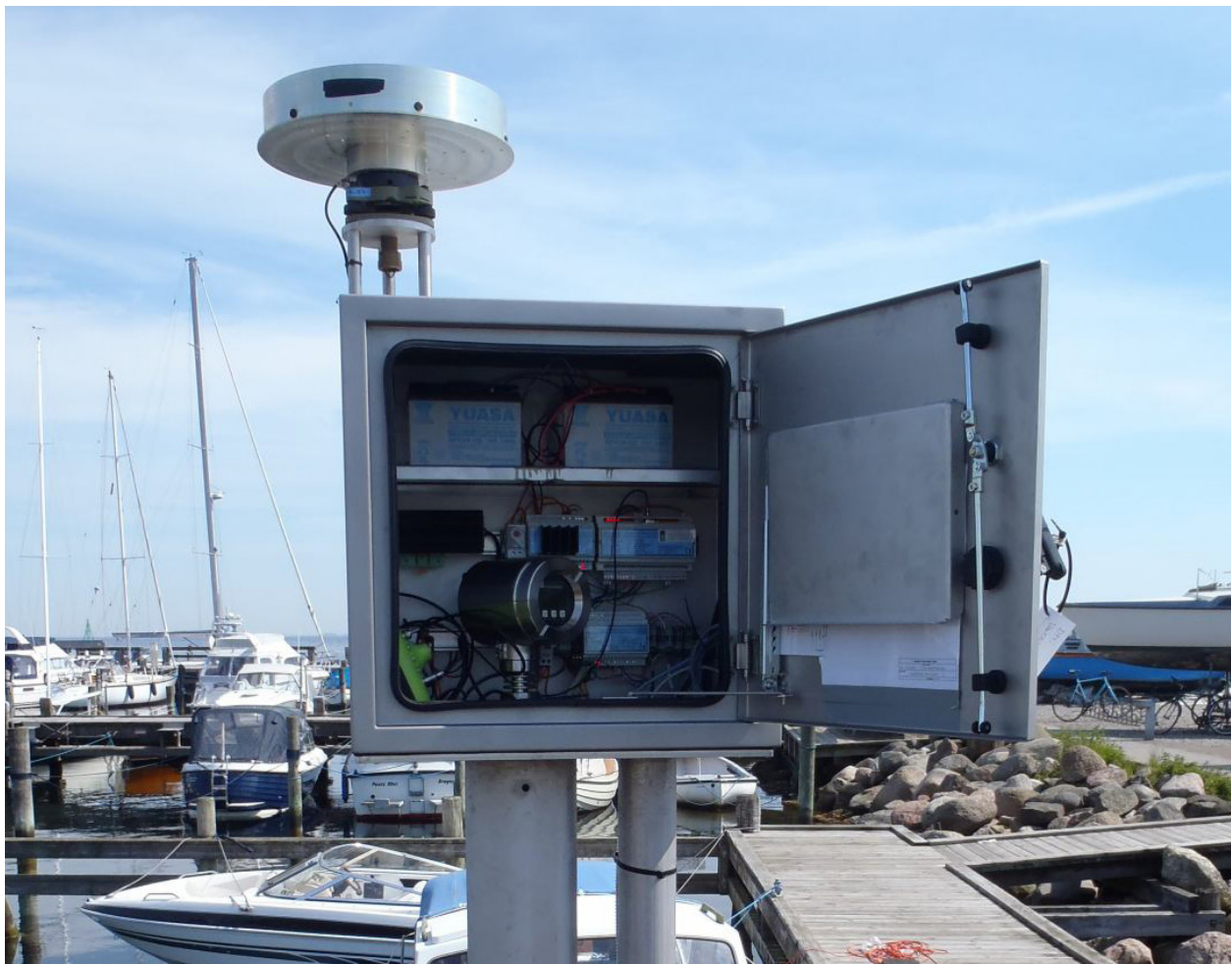
Figure 4.6 An installation at Dragør, Denmark. On the left can be seen an Endress+Hauser radar gauge mounted on top of a stainless steel tube (approximately 17 cm diameter) that functions as a stilling well and waveguide. This tube has an end cap with a 30 mm diameter inlet. Inside the tube is a filter to prevent biological intrusions. At the top of the tube are 4 holes with filters to prevent condensation on the radar antenna. On the right is a stainless steel tube containing pressure sensor cables. (Photograph Danish Meteorological Institute).
