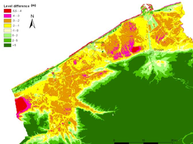
Fig. 1. Level difference between land and North Sea during an average yearly storm of 5,5m TAW (edited from Verwaest et al., 2005)
