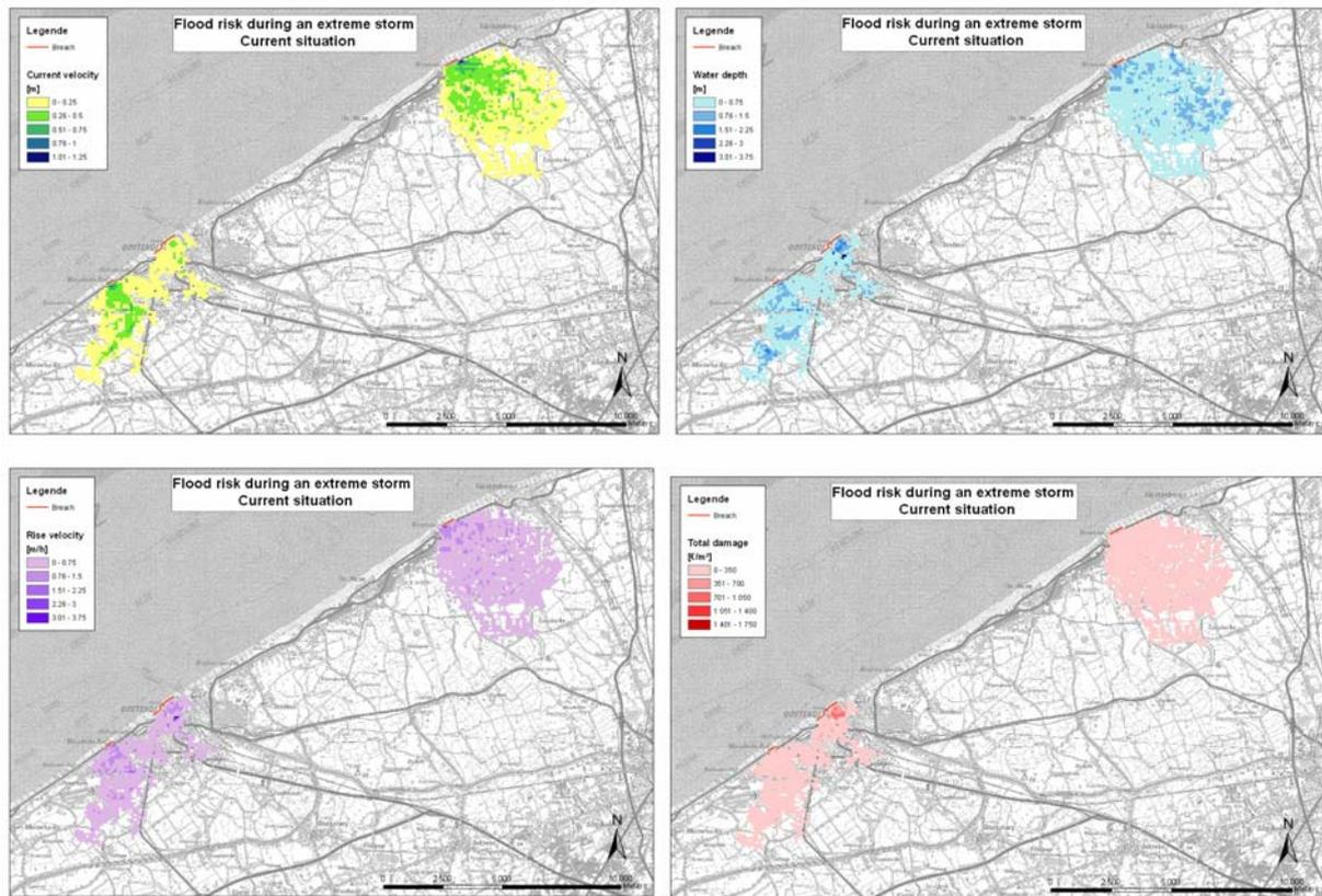
Fig. 3, 4, 5, 6. Flood risk calculations for an extreme storm under present climate conditions: current velocity [m/s], water depth [m], rise velocity [m/h] and total damage [€/m<sup>2</sup>].
