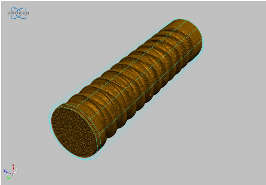
Figure 2: Geometric Figure Volume (GFV) obtained calculating the volume of the cylinder that inscribes the probe.
