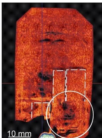
Fig. 3. X-ray microtomographic image of a section of the ADP-KDP crystal grown from solution with ADP:KDP = 80:20 (% w/w). The solution was not stirred. The white circle denotes the area of the crystal splitting.
