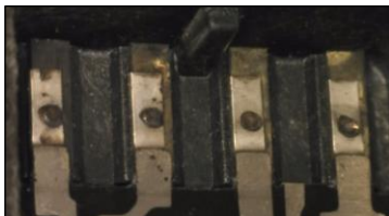
Figure 1. Weld joints between connectors and lead frame
