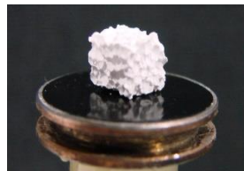
Figure 1. Biomaterial from Ceraver, Calciresorb bone like ®
