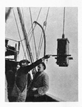
The apparatus consists of a quadrangular tube of iron  $(20\times20$  cm.) which is lowered by wire from the ship. The moment it touches the bottom it is driven into the soil by the impact of a heavy weight (20 to 40 K2) which slides along
