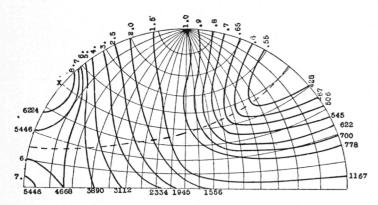
Fig. 9. Distribution of sky brightness with a cloudless sky and the sun  $40^{\circ}$  above the horizon. (The position of the sun is indicated by x.) A stereographic projection of the half of the sky on one side of the sun's vertical. The figures at the top give the brightness relative to zenith brightness; the figures at the opposite ends of the lines of equal brightness give the brightness in millilamberts. (After Physics of the Earth — 3, Meteorology, p. 56.)
