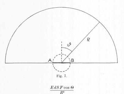
Integrating over the hemisphere and putting the total light flux proportional to the reading of the galvanometer  $U_h$ , the factor of proportionality being C, we get
