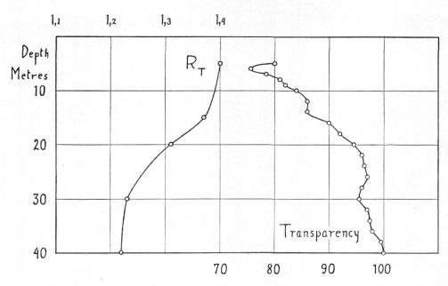
Fig. 11. The factor  $R_t$  as function of the depth and the transparency of the water. (Experiments 5 and 6.)
