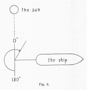
with the photometer directed towards the ship were avoided, as they were influenced by the shadow of the ship. For this reason measurements were only taken over a range of about 210° on the horizontal scale. However, plotting the light vectors in a central vector diagram the enveloping curves should be symmetrical to the direction through the sun and it is therefore permissible to extrapolate for the missing angles.
