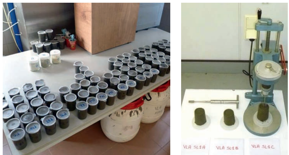
Figure 14. Engineered sediments during hardening and the laboratory vane apparatus.
