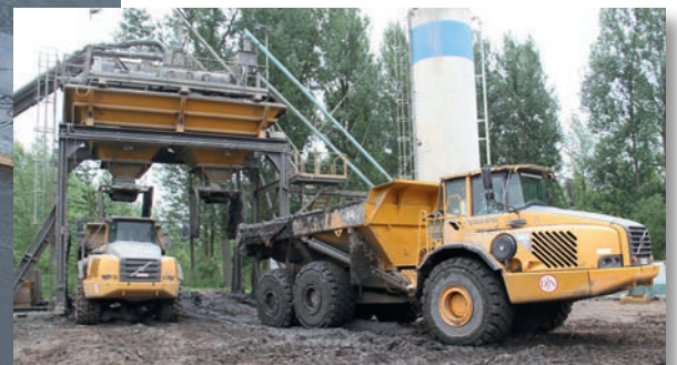
Figure 18. Sediment-additive mixing unit where the sediments are 'engineered'.
