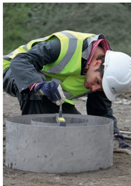
Figure 25. Double ring infiltrometer for permeability testing.
