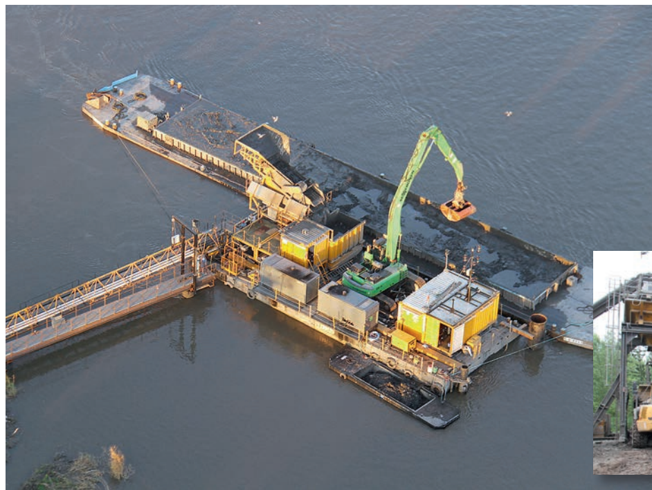
Figure 17. A specially designed discharge pier accommodates the high tidal amplitude and strong currents at the site. A long-reach excavator unloads sediments from a barge and places them over a vibrating sieve. The high-density, sieved material is then pushed through a pipeline towards the mixing unit.
