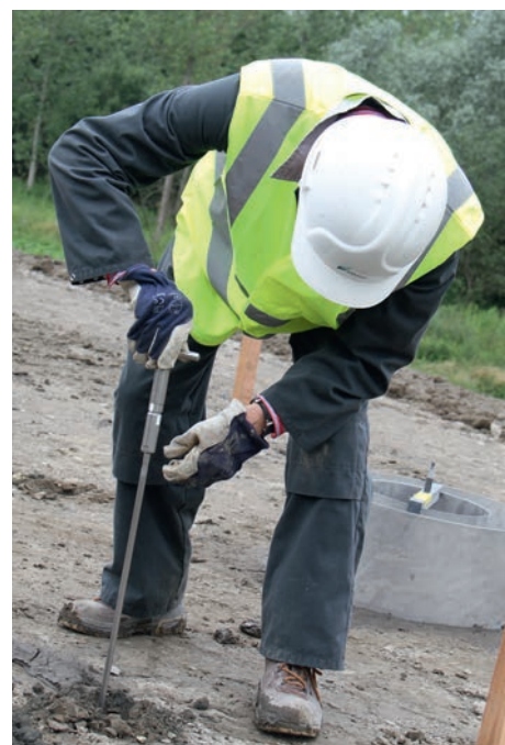
Figure 24. Hand vane for shear strength testing.
