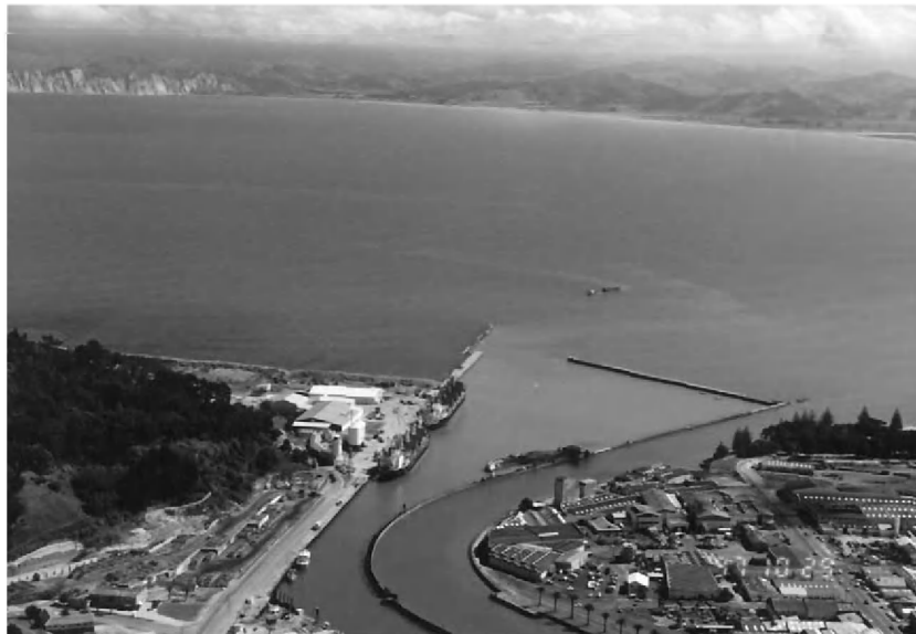
Fig. 2. Aerial view of Port Gisborne navigation approach channel, log handling area and existing breakwaters. Additional reclamations are envisaged along the shore platform to the east (left of photo).
