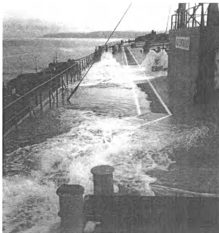
Figure 3 Ballast-water exchange using the tank overflow technique, in which the tank is flushed out by pumping through three times its volume of seawater.
