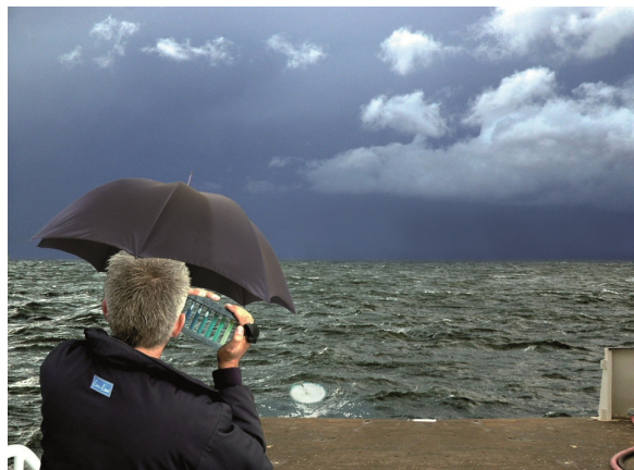
Figure 4.4 - A Forel-Ule observation is taken, at the shady side of the vessel, above a submersed Secchi disc, with the disc lowered to a depth of approximately half the Secchi disc depth. The reading of the scale should be done in the shadow.
