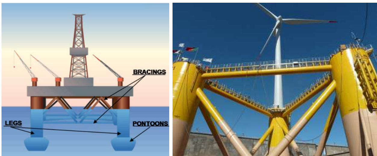
Figure 15. Semi-submersible structure. (a) Semi-submersible structure concept for Oil&Gas. (b) WindFloat Concept for wind energy.
