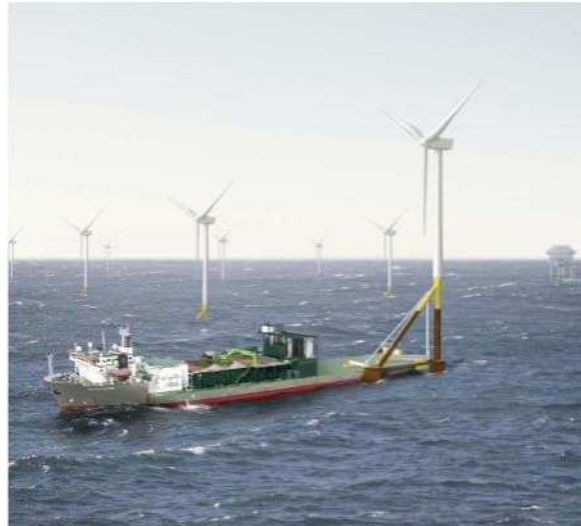
Figure 60. SPT Offshore self-installing wind turbine (URL 15)
