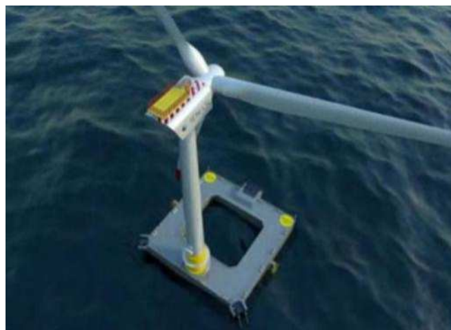
Figure 52. Ideol floating foundation by Ideol Offshore (URL 6)
