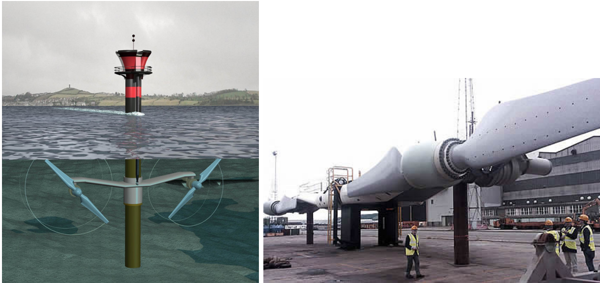
Figure 73. Seagen generator (Source: Alternative Energy, 2007, MetaEfficient, 2008).
