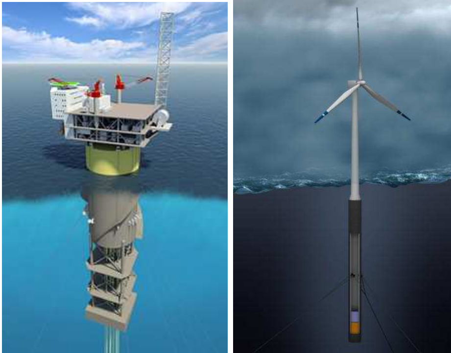
Figure 17. The SPAR concept. (a) Statoil concept (Aasta Hansteen field, 2012). (b) HyWind (Statoil)
