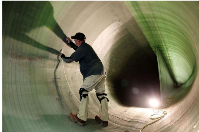
FIGURE 3.2 A quality inspector examines the interior of a wind turbine blade at the Siemens Wind Turbine Blade. Source: AP Photo/The Hawk Eye, John Lovretta
