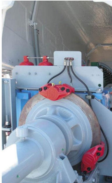
FIGURE 3.13 A typical wind turbine brake. Source: http://www.windpowerengineering.com
