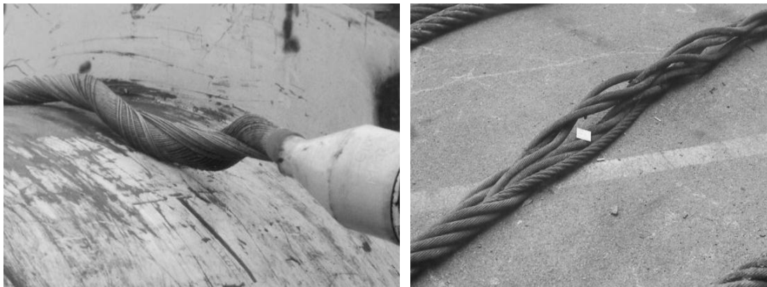
Figure 5.4 - Typical failure modes (Chaplin 1998). Left: a coiled wire damage due to high torque load. Right: Slipping damage of a six-strand cables.
