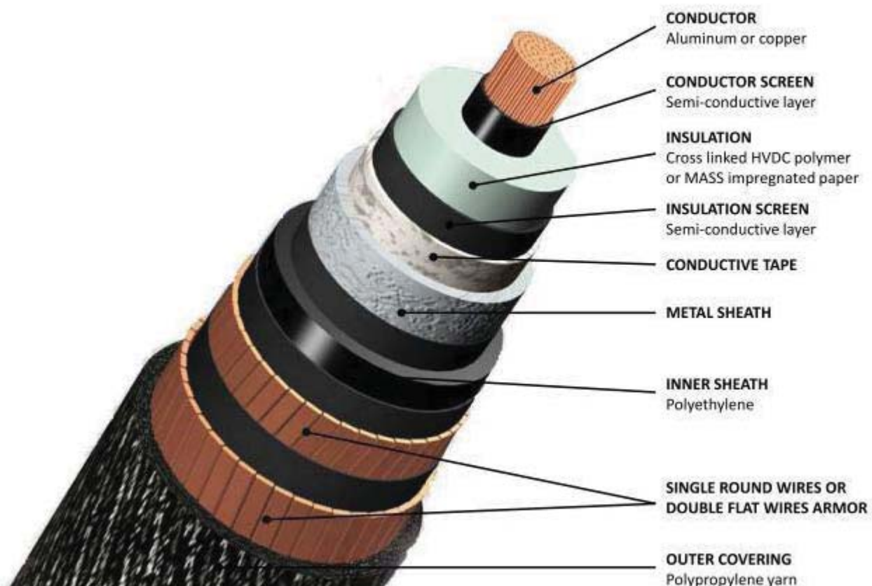
Figura 40 - Single core submarine cable, AC or DC [source: Europacable].
