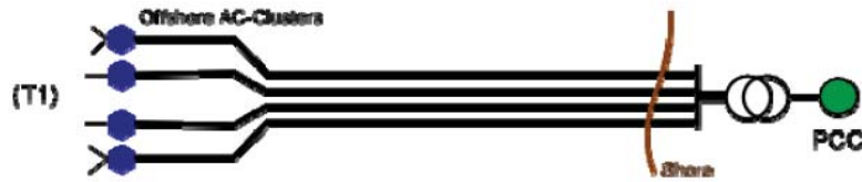
Figure 6 - Basic concept of transmission system for small marine farms [6].
