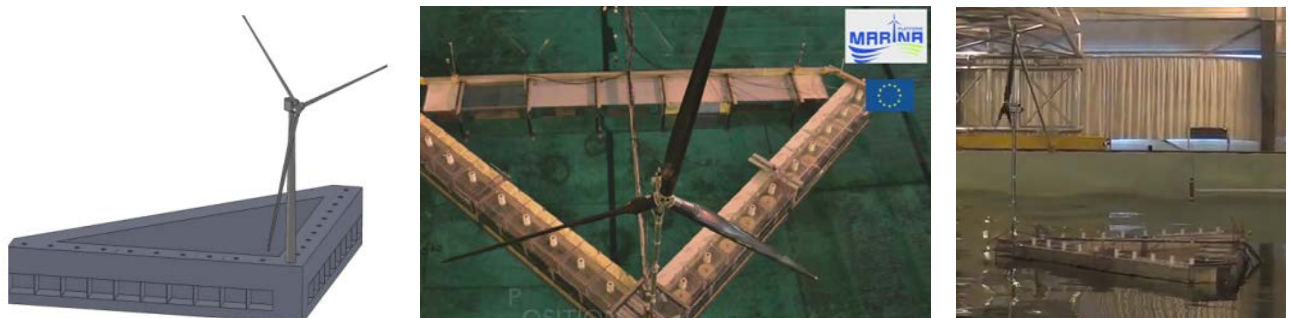
Figure 7. Marina platform: Large semi-submersible - Wind Turbine + multiple OWC [7].
