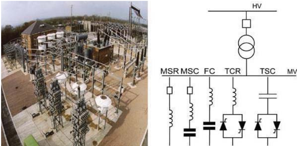
Figura 52 - SVC configurations [source: Alstom]
